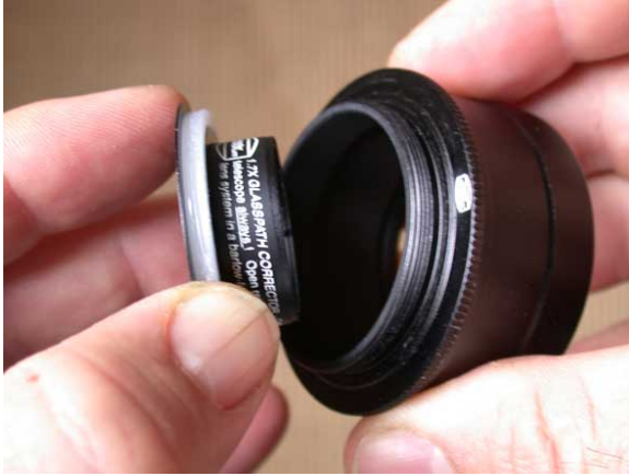
Figure 3 This picture shows how to insert the Glasspath Compensator into the T2 2" nosepiece. The included white plastic ring must be pressed onto the compensator threads in order to center the compensator within the nosepiece adapter.
