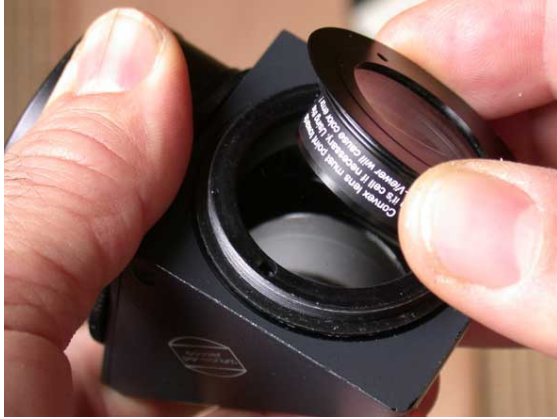
Figure 10 Threading the Glasspath Compensator into the top of the various Baader T2 diagonals.
