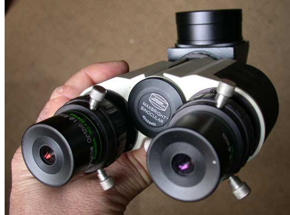
Figure 11 Maxbright Binoviewer with Zeiss prism diagonal (T2-1B) and 2" nosepiece (T2-16).
