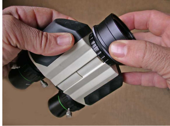
Figure 4 After placing the Glasspath Compensator into the 2" nosepiece, screw the nosepiece onto the threaded T2 ring on the front of the viewer, turning the ring until tight.
