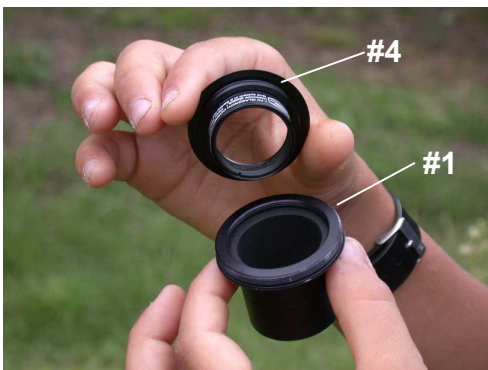
Figure 2 Glasspath Compensator used with 1.25" nosepiece. Compensators may also be used with many other Baader T-2 accessories.
