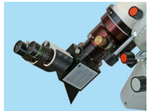
Figure 11 Maxbright binoviewer, attached directly onto the Herschel Solar Prism with T2-27 Adapter 2"/T2.
