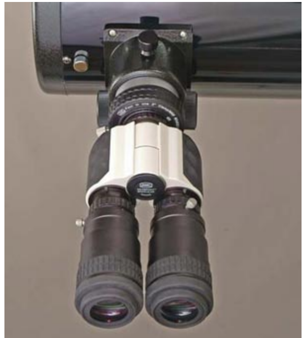
Figure 6 Maxbright Binoviewer and 2" Newtonian 1.7x Glasspath Compensator in 2" Focuser of a Newtonian Telescope
